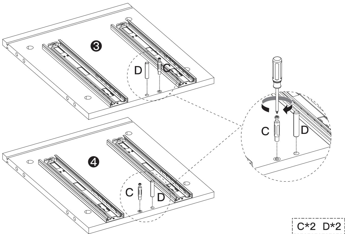
**STEP 6** Slide Part 3 and Part 4 into Part 18 as shown below. Insert [F] into part 18 and tighten with Phillips Screw Driver to secure the assembly together.
