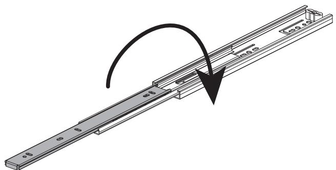
3-3 Move release trigger as shown below while pulling on Drawer Side.
