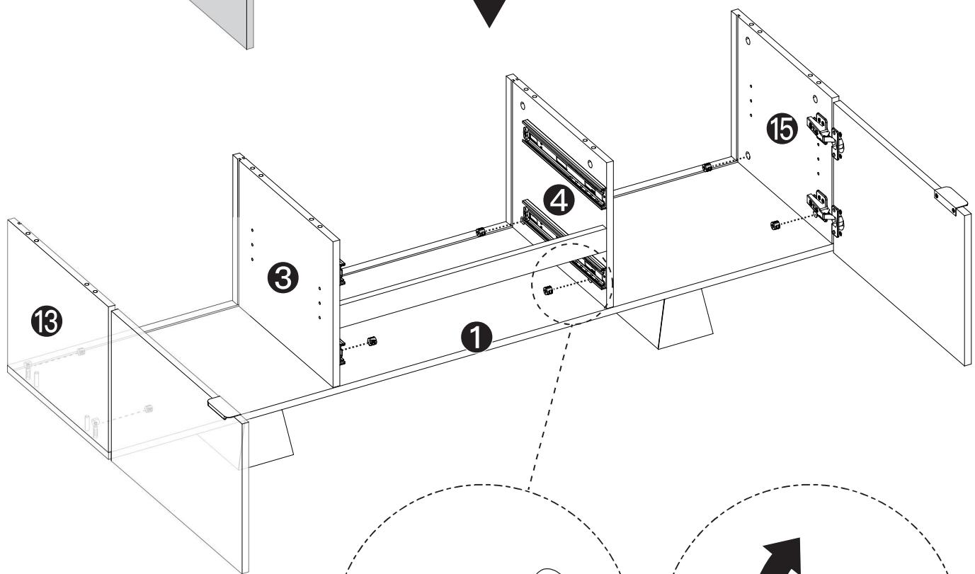
Insert [F] into Part 3, Part 4, Part 13 and Part 15 as shown below. Tighten with Phillips Screw Driver.
