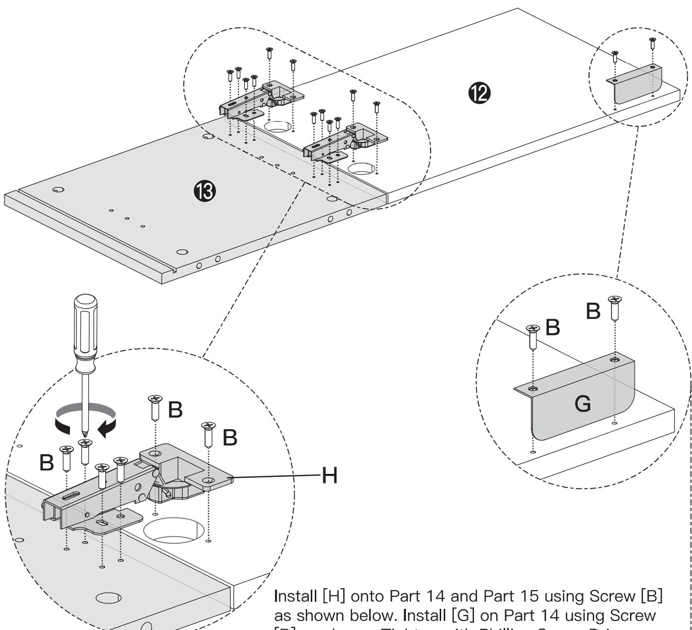
Install [H] onto Part 14 and Part 15 using Screw [B] as shown below. Install [G] on Part 14 using Screw [B] as shown. Tighten with Phillips Screw Driver.
